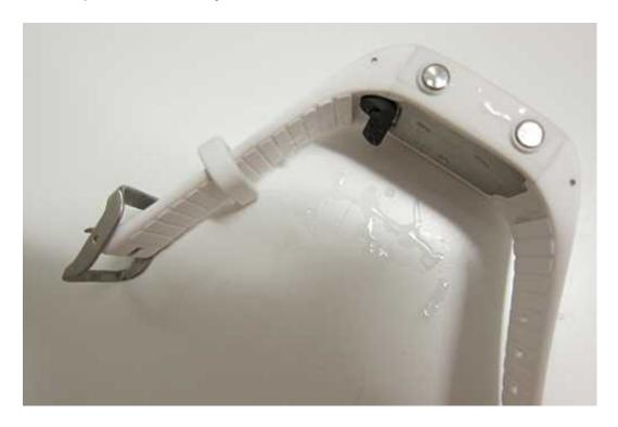
When using the USB port, check that there is no moisture, hair, dust or dirt on the sealing surface area. Gently wipe off any dirt. A toothpick can be used to remove hair, dust or other dirt from the connector cavity. Don't use any sharp tools for cleaning to avoid scratching.
