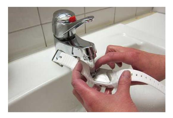
3. After rinsing, leave the cover open for a while to let the USB port dry. **Do not charge the M400 when the USB port is wet or sweaty**.
