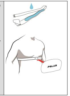
Detach the connector from the strap, and rinse the strap under running water after every training session. Sweat and moisture may keep the heart rate sensor activated, so also remember to wipe it dry.
