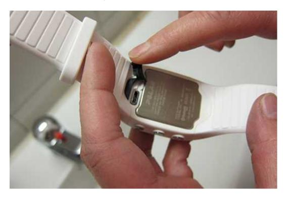
2. Rinse the USB port with lukewarm tap water. The USB port is water resistant and you can rinse it under running water without damaging the electronic components.
