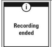
2. To stop a training session, press and hold the BACK button for three seconds during training recording or in pause mode until **Recording ended** is displayed.
